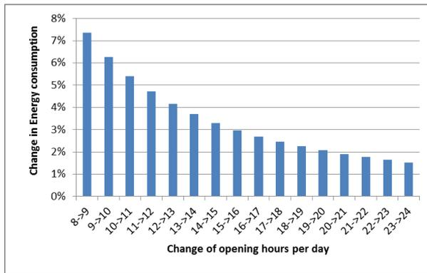
Figure 31: relative energy consumption change per additional opening hour, as evaluated from the new PI based on CF
