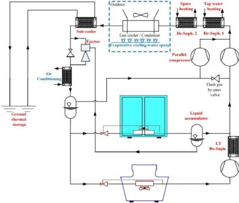
Figure 62: CO<sub>2</sub> booster system with a number of state of the art options to increase energy efficiency
