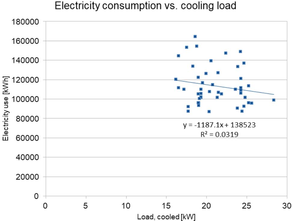
Figure 66: Refrigeration system electricity consumption as function of nominal chilled load.
