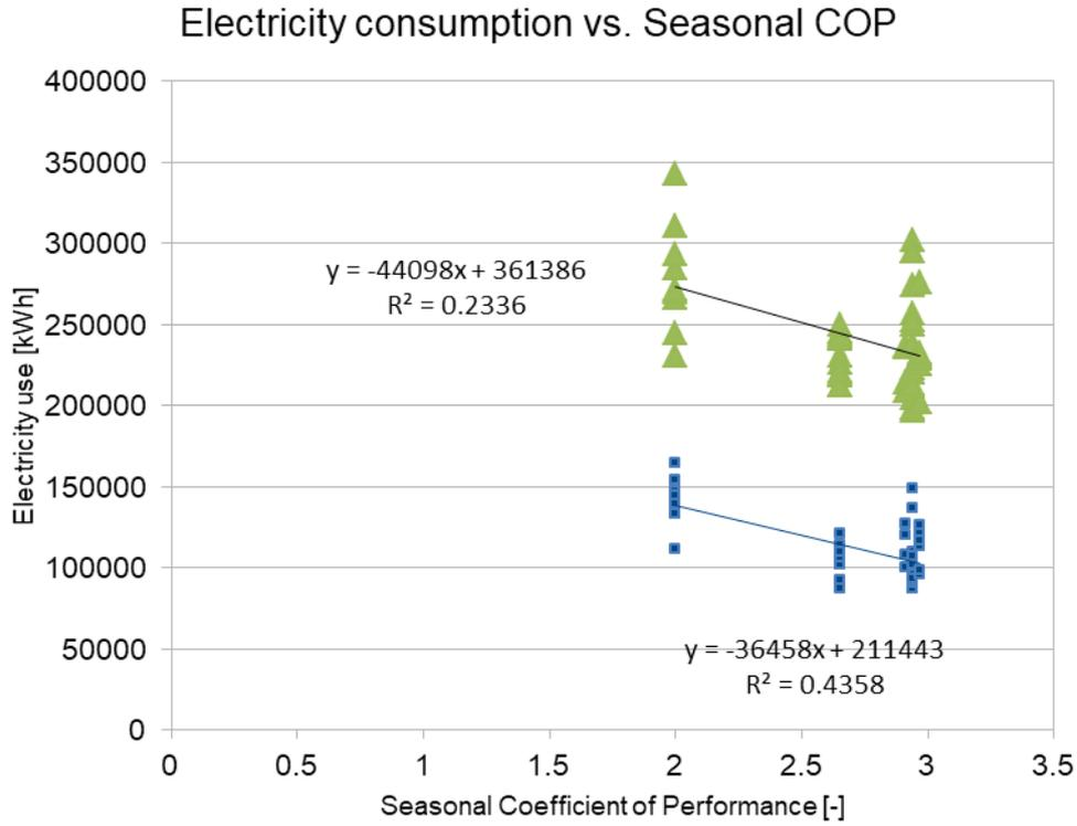
Figure 72: Electricity consumption as function of Seasonal Coefficient of Performance (SCOP). Blue square is refrigeration; green triangle is total
