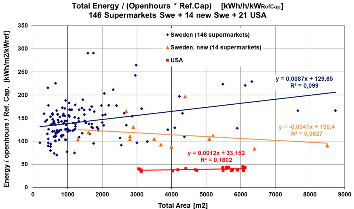
Figure 38: graphical evaluation for the proposed performance indicator “Total energy consumption / (opening hours \* installed refrigeration capacity), based on data sets from Annex 31
