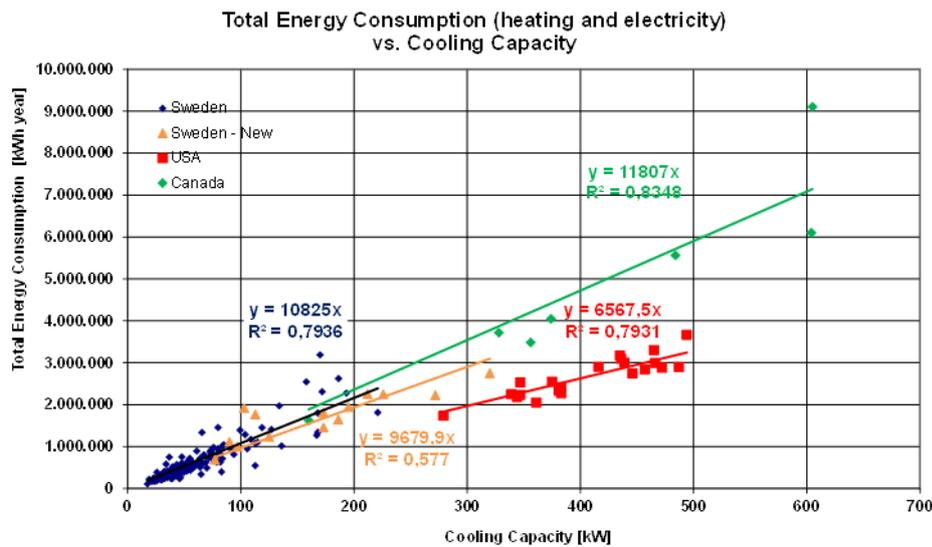
Figure 22: Regressions of total yearly energy consumption with installed cooling capacity for the data set of Swedish, USA and Canadian supermarkets (Annex 31).
