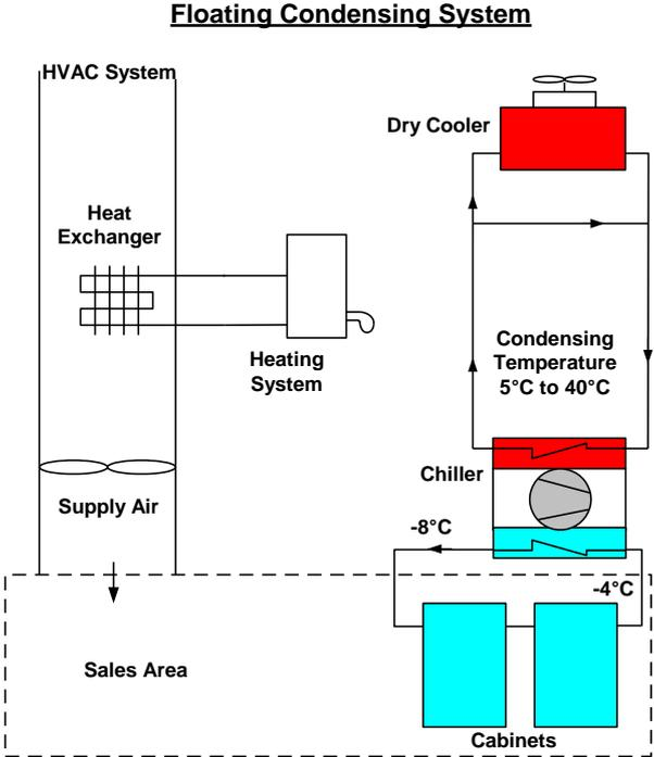
Figure 64:: Floating Condensing System
