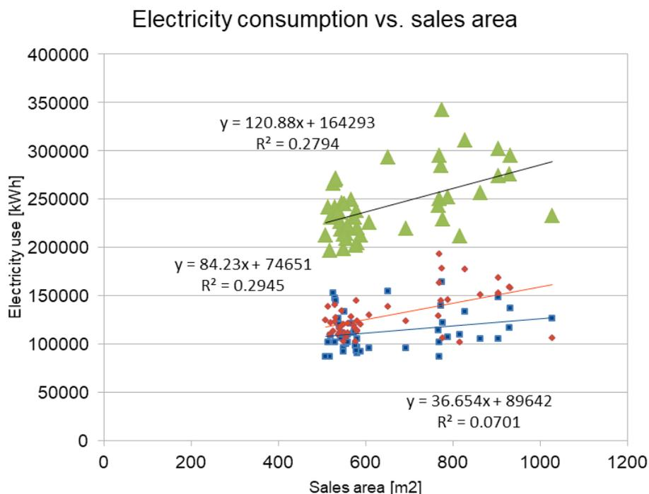
Figure 65: Electricity consumption as function of sales area. Blue square is refrigeration; orange diamond is non-refrigeration; green triangle is total
