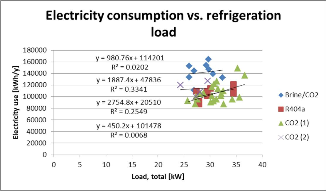
Figure 69: Refrigeration electricity use as function of nominal refrigeration load, grouped by refrigeration system type. Trend line functions in same order as legend
