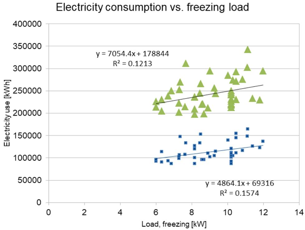
Figure 67: Electricity consumption as function of nominal frozen load. Blue square is refrigeration; green triangle is total
