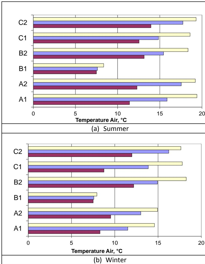
Figure 35: Measured average air temperatures,  $t_{air}$ , at three different heights above the floor and 0.5 m in front of refrigerated display cabinets during summer and winter conditions (data from Lindberg, 2009).
