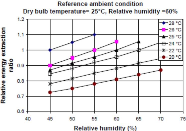
Figure 36. Relative heat extraction rate (cooling load) in a vertical open display cabinet as a function of ambient relative humidity (according to Brolls and diagram from Axell (2002).). For horizontal (island type) cabinets the influence is lower, as well as for cabinets covered by night curtains or glass doors.
