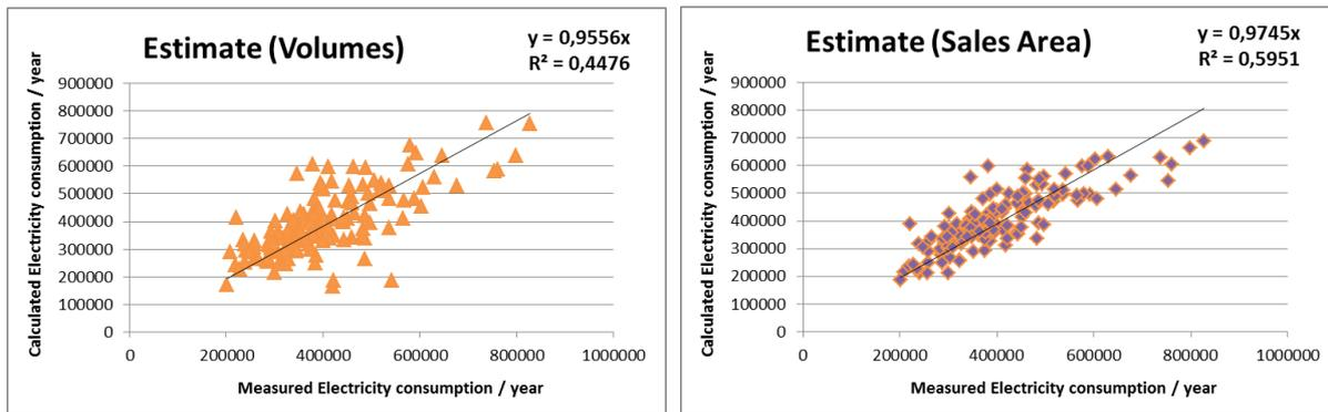
Figure 17: Estimate of yearly electrical energy consumption based on volumes of RDC's and storage cells (left) and based on sales Area (right)
