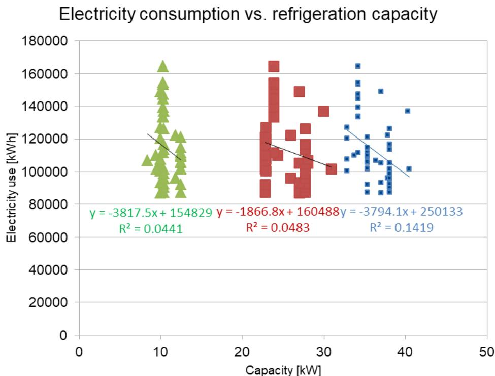
Figure 70: Refrigeration system electricity use as function of installed capacity. Green is LT, red is MT, blue is total refrigeration capacity. Significant clustering per refrigeration system type, due to low or no capacity variation with same system type
