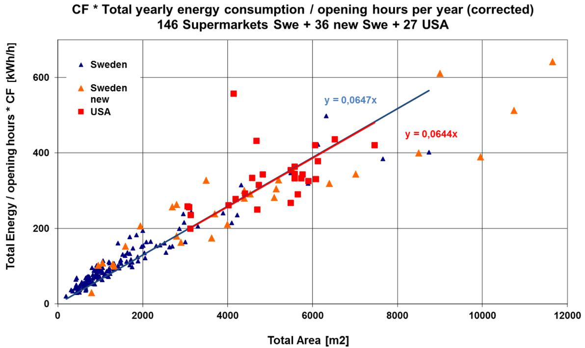
Figure 29: Total energy demand / opening hours with correction factor versus total area for supermarkets in Sweden and USA. Trend lines for 146 Supermarkets SWE (blue line) and 27 USA supermarkets (red line) with coefficients shown.
