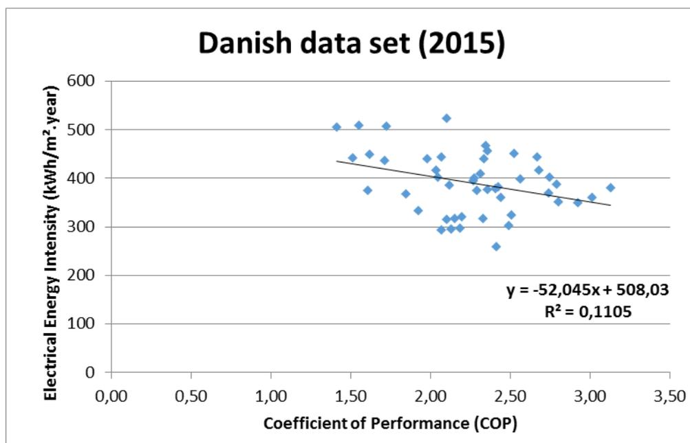
Figure 41: SCOP values calculated on the basis of calculated refrigeration demand and measured yearly energy consumption for refrigeration, for the Danish data set (2015).
