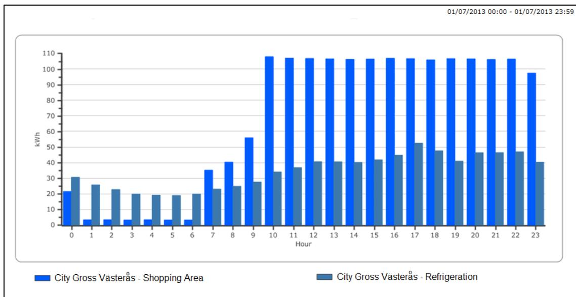
Figure 7: Energy usage in sales area and energy use for refrigeration. Energy use during night hours is strongly reduced in the shopping area, and slightly reduced for the refrigeration system (compared to daytime use). There are doors on the cabinets in the supermarket.
