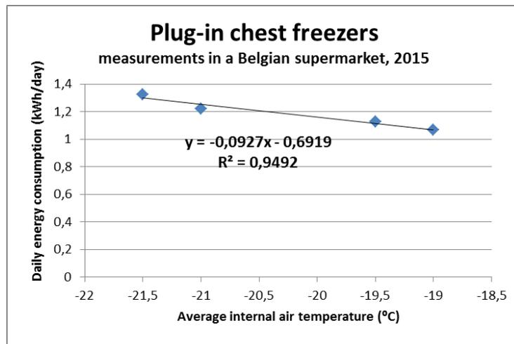
Figure 52: trend line of energy consumption with average internal air temperature for measurements on plug-in chest freezers in a Belgian supermarket (2015)
