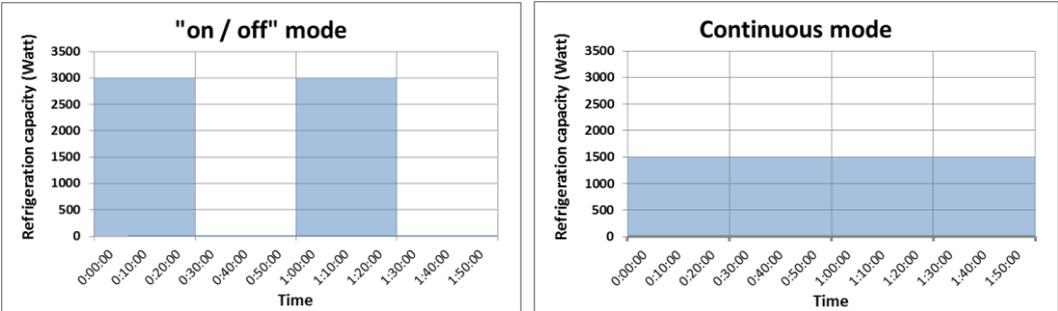
Figure 53: Refrigeration capacity demand as a function of time for a refrigerated display cabinet operated in “on off” mode (left) and in continuous mode (right).
