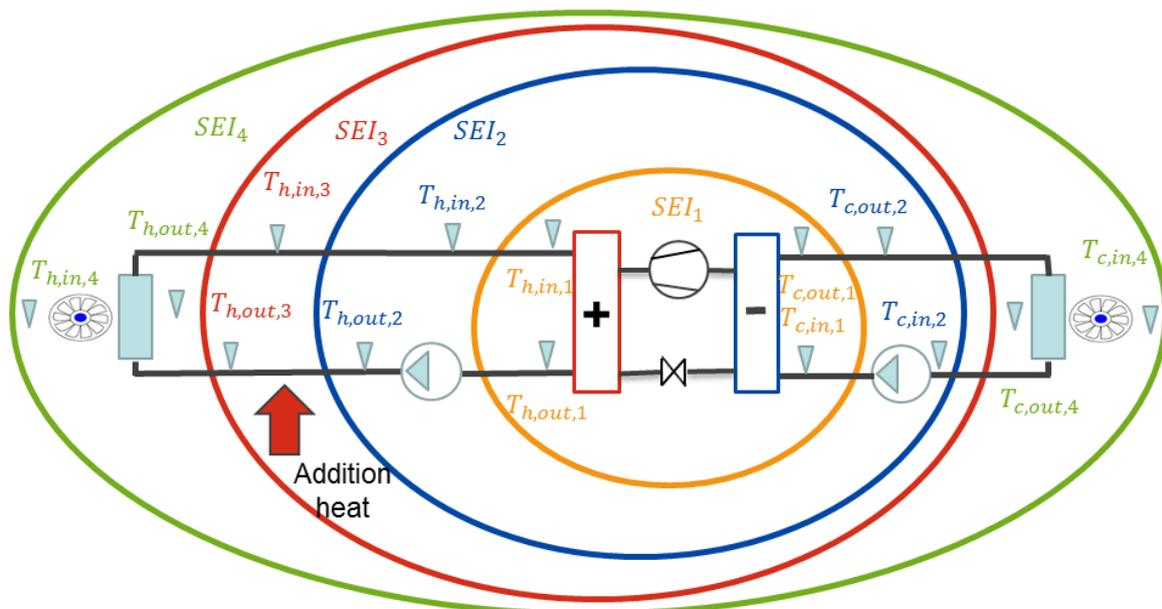
Figure 39 System boundaries used to define SEI1,2,3,4 and reference temperatures  $T_{ref,x,n}$
