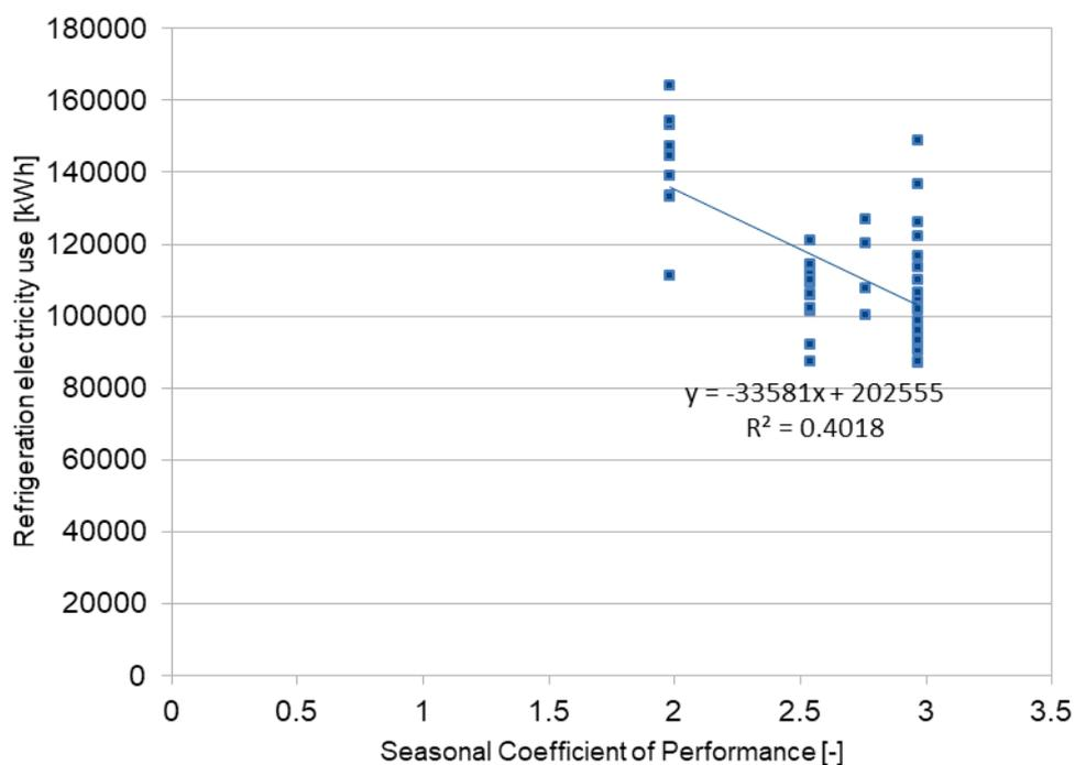
Figure 46: Seasonal COP values calculated with Pack Calculation Pro from refrigeration system specifications, for a reference nominal load of 9 kW at LT and 21 kW at MT, representative for the Annex 44 data set for Denmark (2015), for the four refrigeration system types in that data set.
