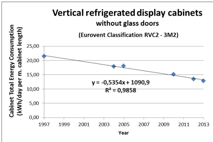
Figure 48: trend in energy use of vertical refrigerated display cabinets, based on the analysis of a large collection of cabinets offered on the market by different (EU) manufacturers (from H.Moons, 2014).
