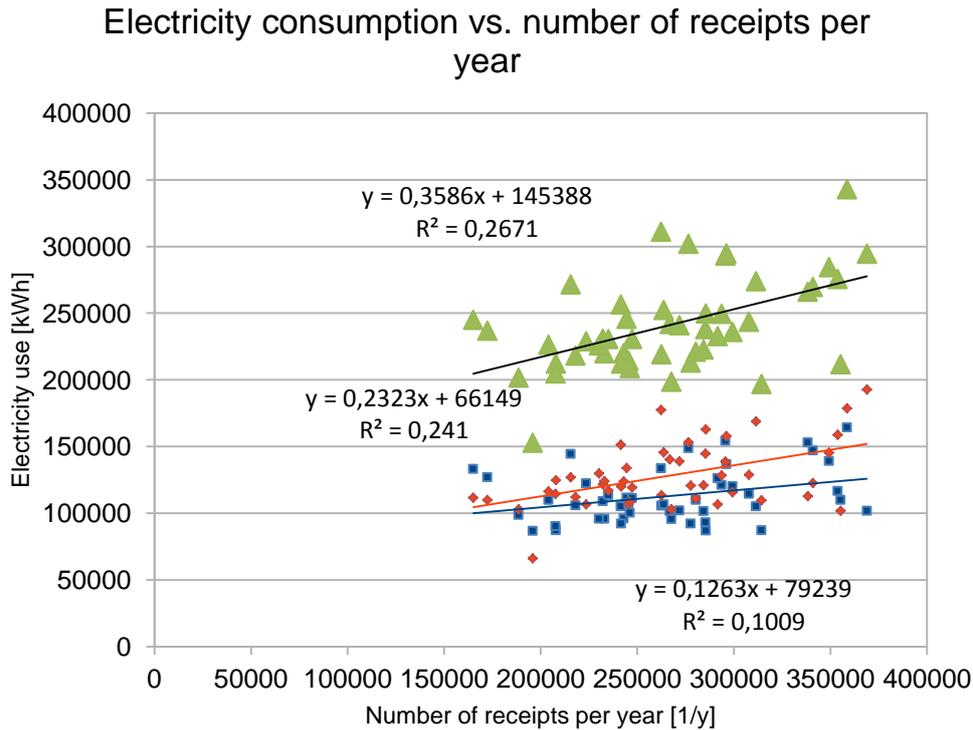
Figure 74: Electricity consumption as function of number of receipts per year. Blue square is refrigeration; orange diamond is non-refrigeration; green triangle is total
