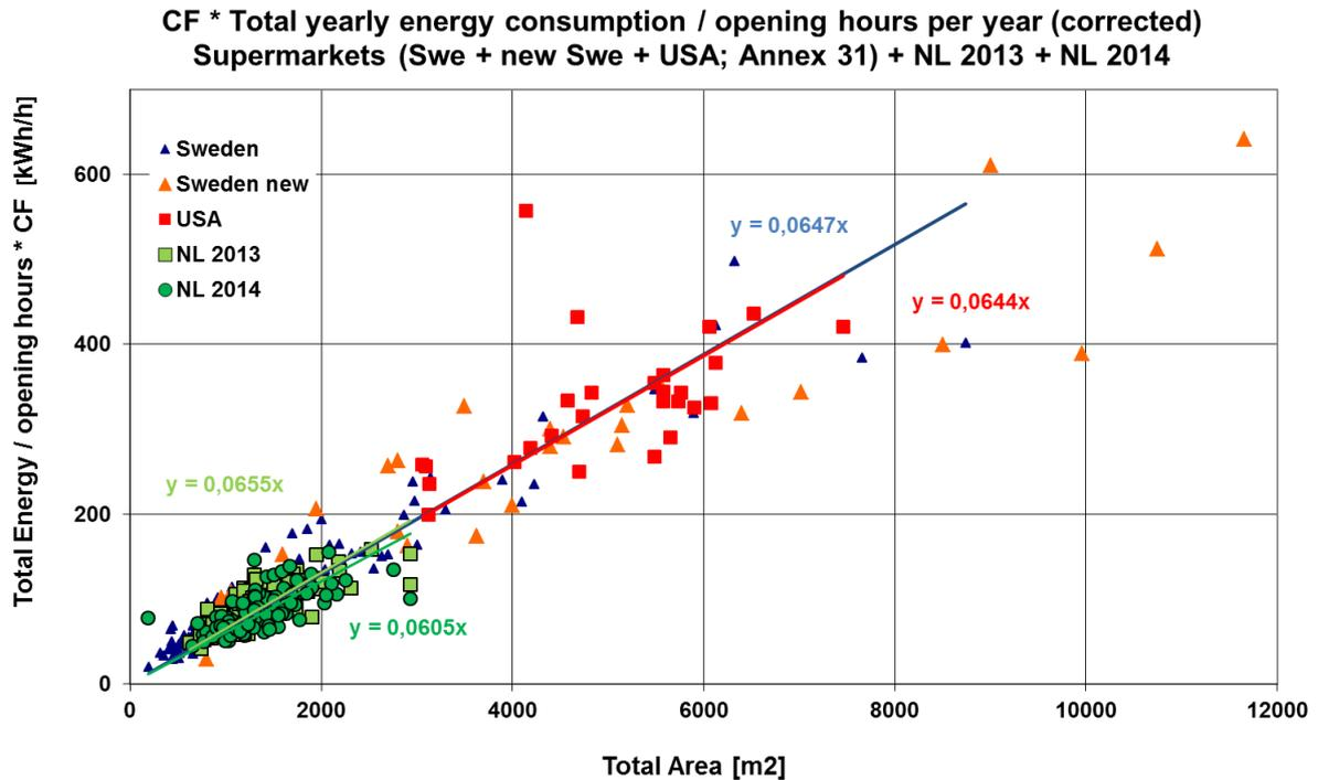
Figure 30: Total energy demand / opening hours with correction factor versus total area from supermarkets in Sweden USA and Netherlands. Trend lines for 146 Supermarkets SWE (blue line) and 27 USA supermarkets (red line) with coefficients shown. Additional trend lines and coefficients are shown for NL 2013 (light green) and NL 2014 (dark green).
