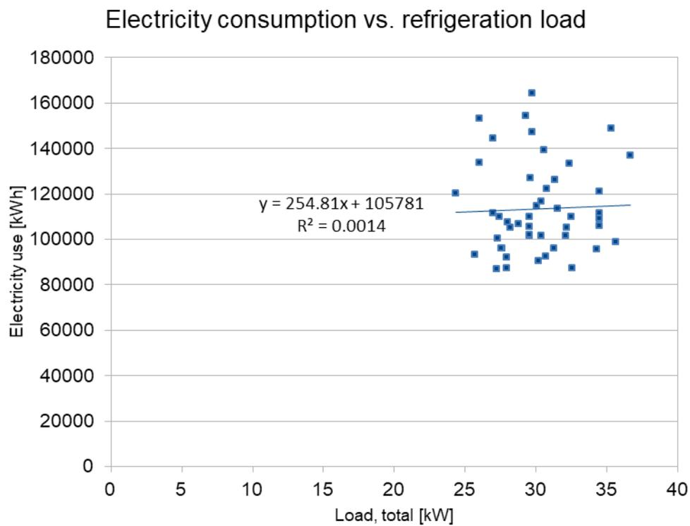
Figure 68: Refrigeration electricity consumption as function of nominal refrigeration load
