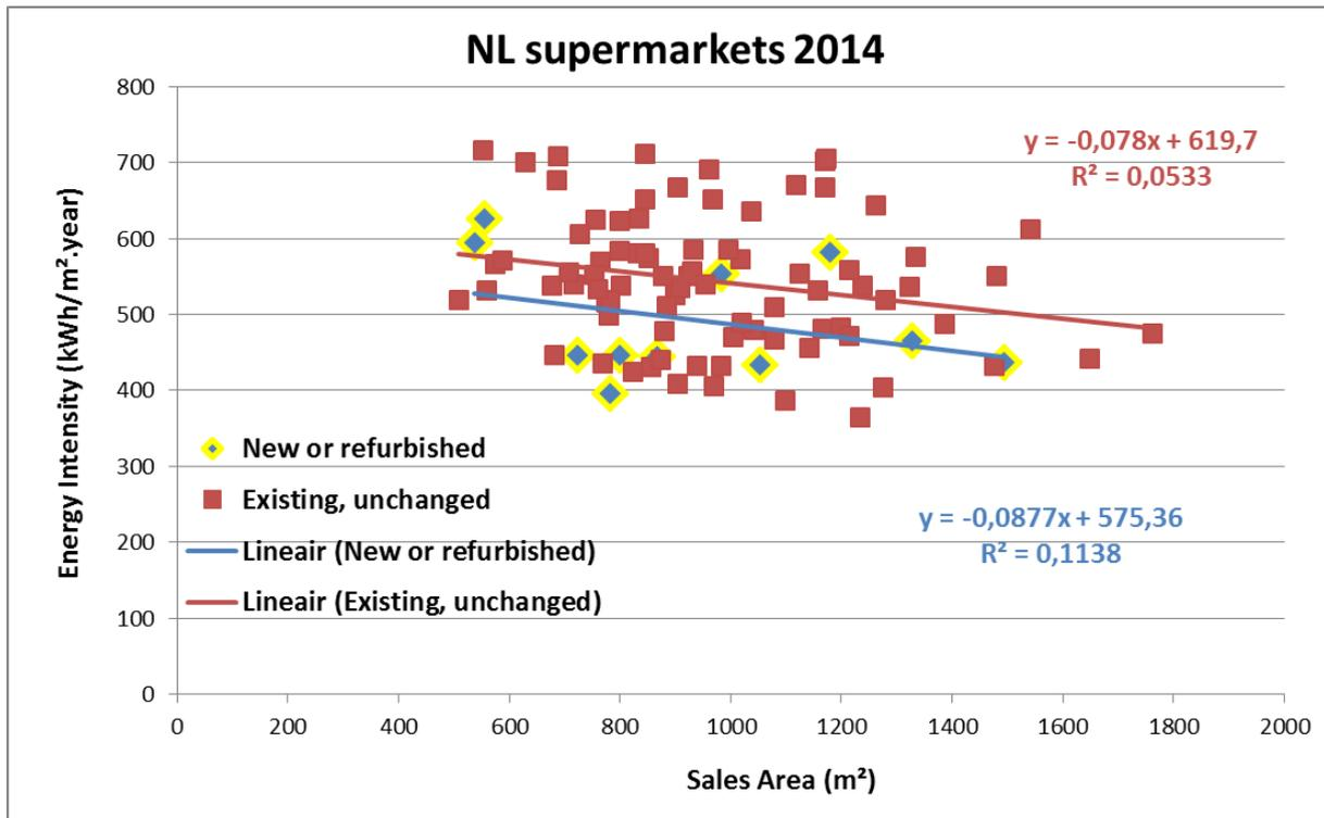
Figure 50: Energy Intensity for the Annex 44 database for The Netherlands (2014), split between unchanged supermarkets and new or refurbished supermarkets – with associated trend lines.
