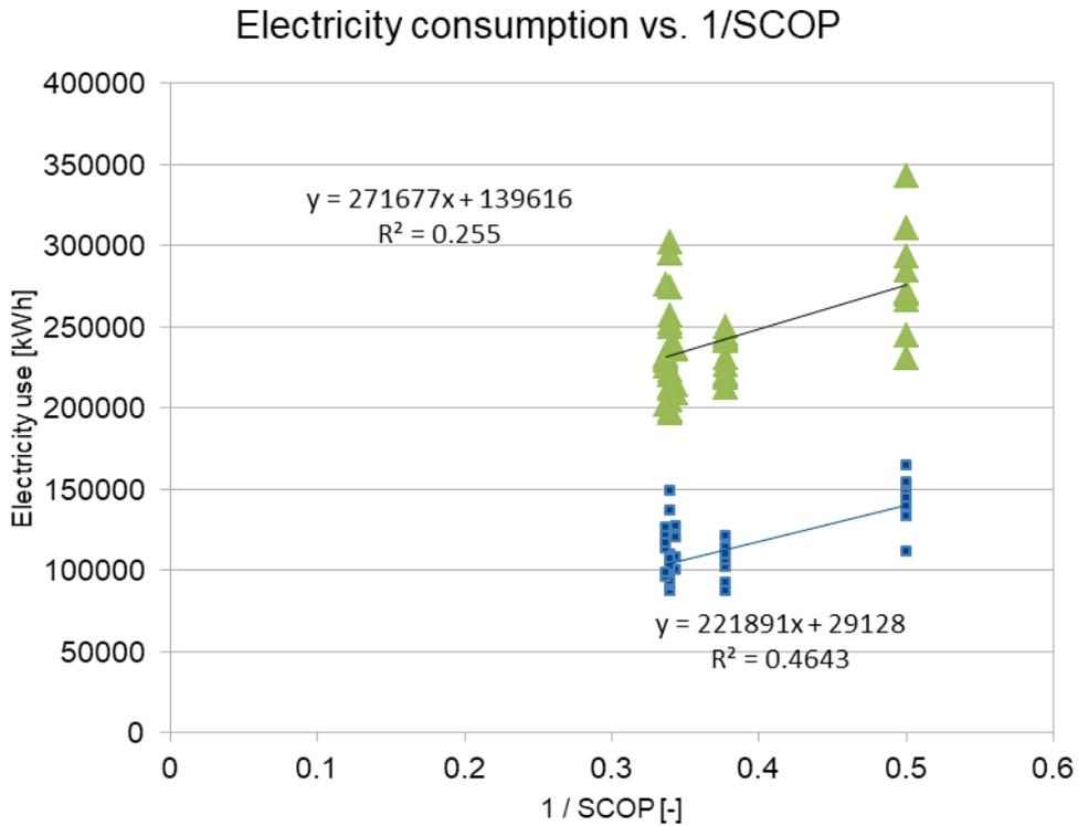
Figure 73: Electricity consumption as function of the inverse of SCOP. Blue square is refrigeration; green triangle is total
