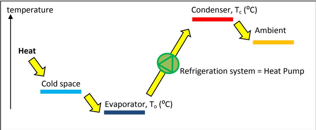
Figure 4: heat leaks into the cold space, is absorbed by the evaporator and pumped to a higher temperature by the refrigeration system. From the condenser the heat flows to ambient.
