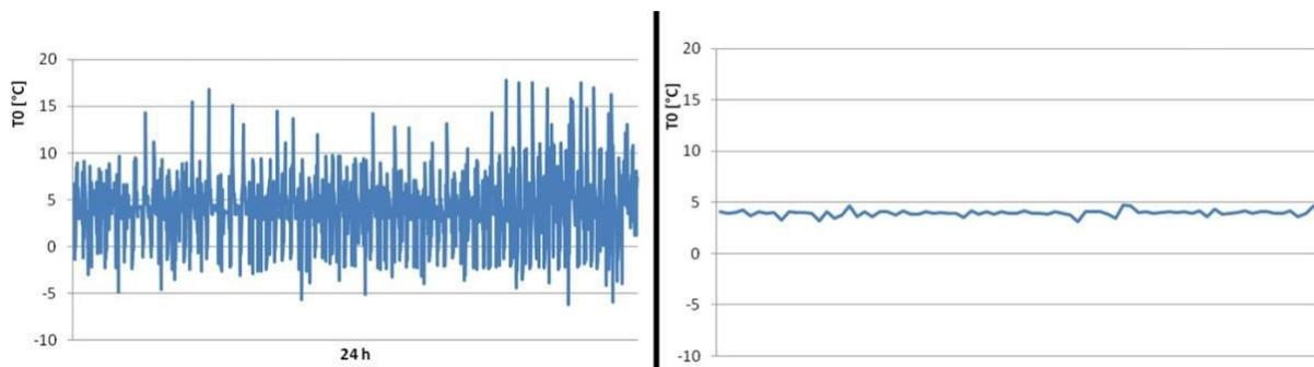
**Figure 54: dynamic evaporation temperature profile before and after a small adjustment to the compressor rack control (from S. Capanelli, 2017).**
