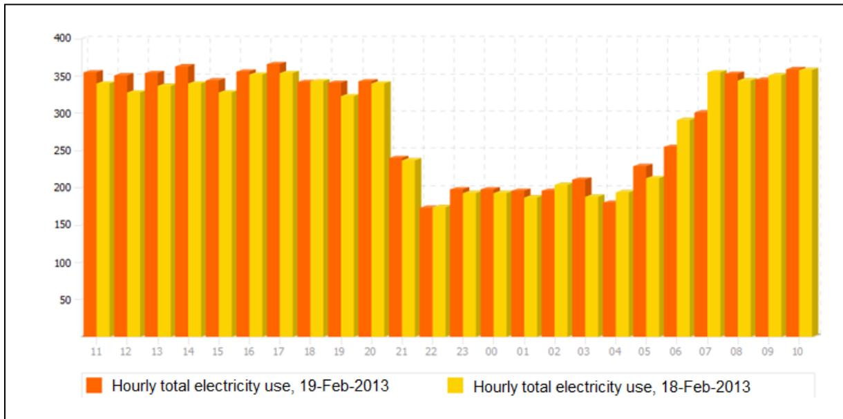
Figure 8: Example of diagram in monitoring system comparing total electricity usage per hour for the days 18<sup>th</sup> and 19<sup>th</sup> of February for a supermarket.
