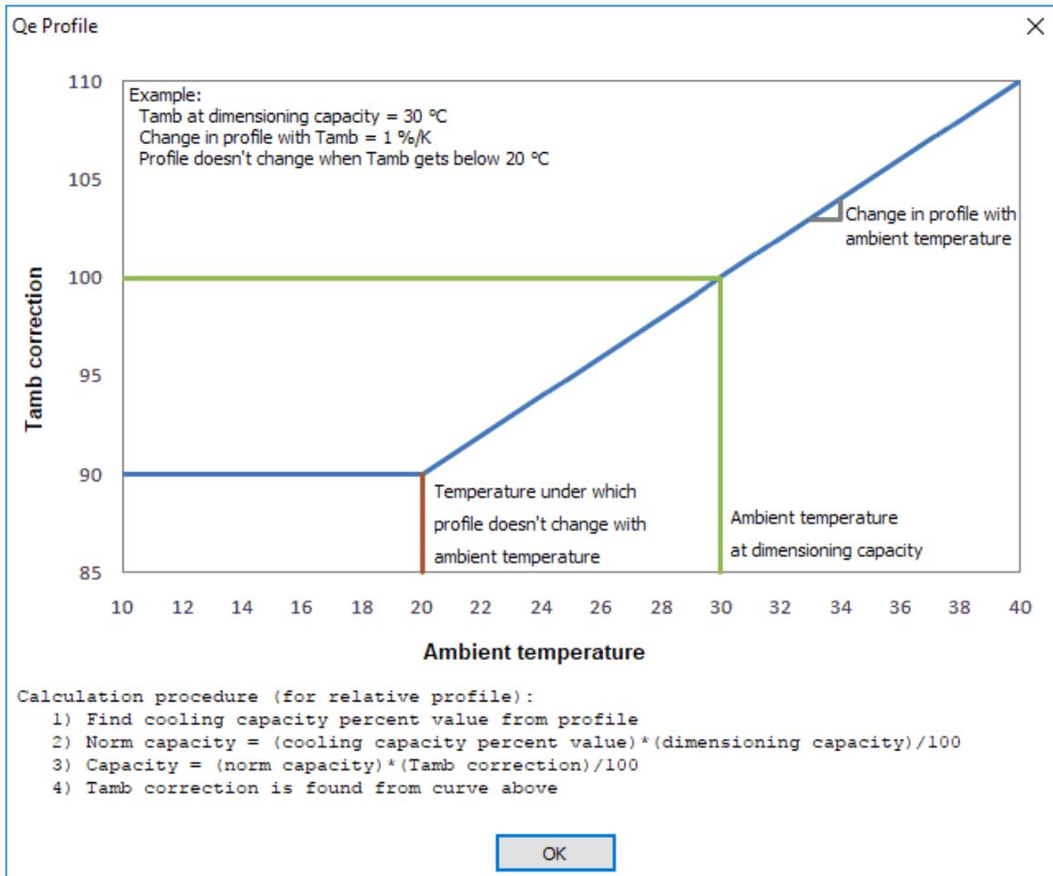
Figure 45: Cooling capacity change with change in ambient temperature. The ambient temperature at dimensioning capacity is 32 °C, the load change with ambient temperature is 1%, and the profile doesn't change further if ambient temperature is below 20 °C
