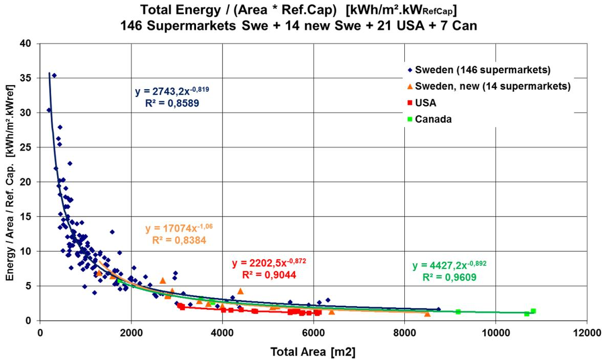
Figure 37: graphical evaluation for the proposed performance indicator “Total energy consumption / (total area \* installed refrigeration capacity), based on data sets from Annex 31.
