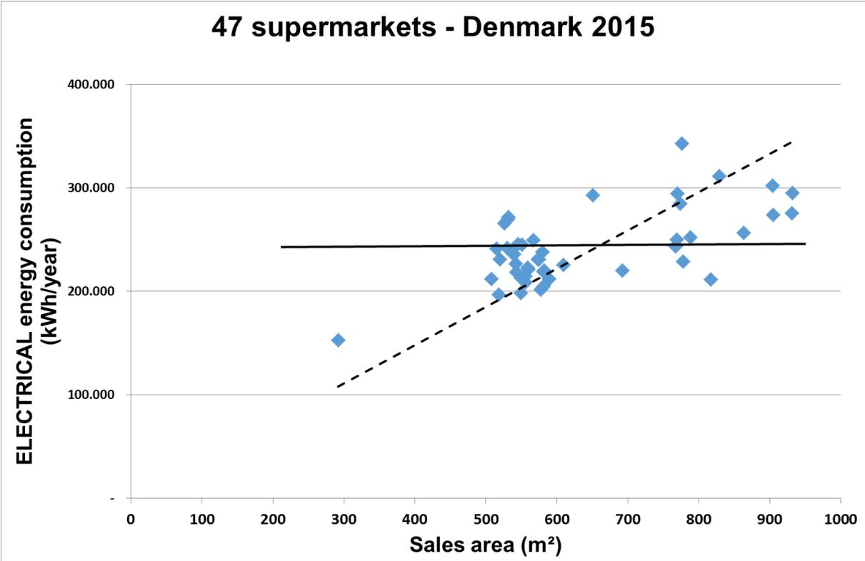
Figure 15: representation of the Danish data set, total yearly electrical energy consumption vs. sales area. The trend line is not shown (only dashed), since a constant value explains the data better than the trend line through the origin (negative R<sup>2</sup> value).
