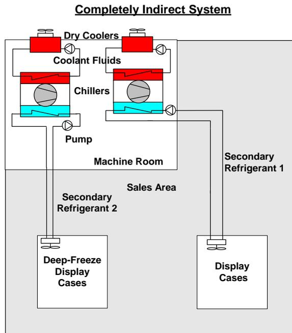
Figure 56: Completely Indirect System (Arias, 2005)
