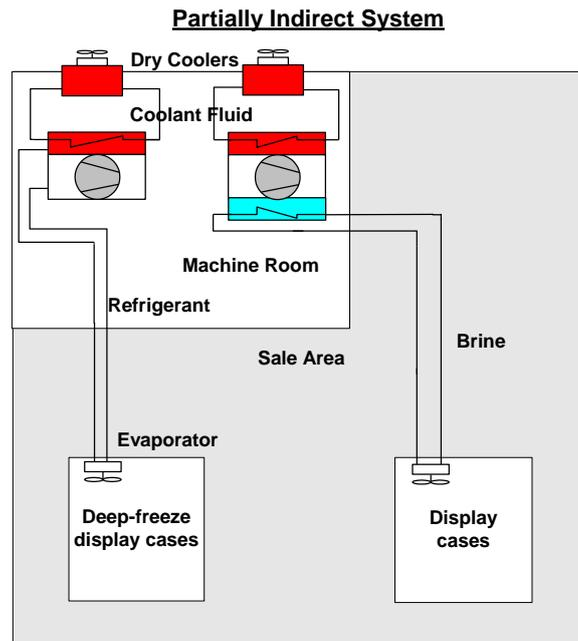
Figure 57: Partially Indirect System (Arias, 2005)
