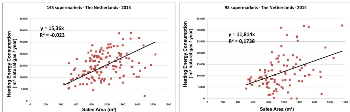
Figure 14: representation of the Dutch data sets: heating energy consumption versus Sales area (2013 and 2014).
