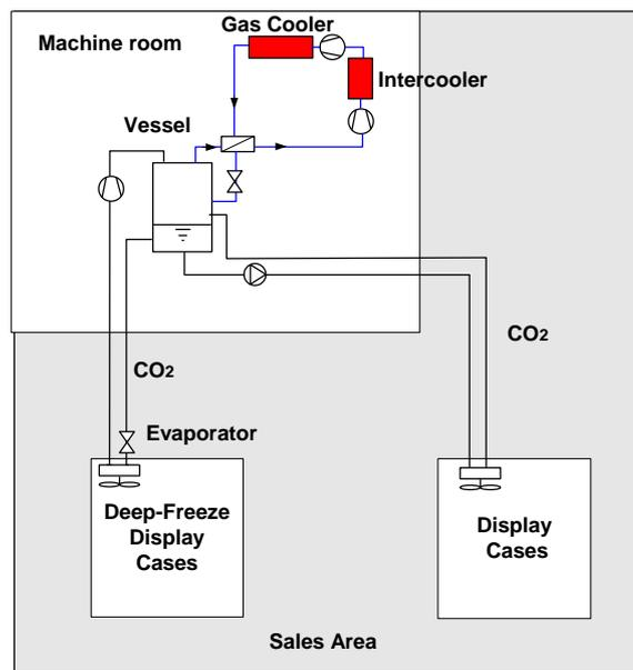
Figure 60: Multistage System 1 with CO<sub>2</sub> (Arias, 2005)
