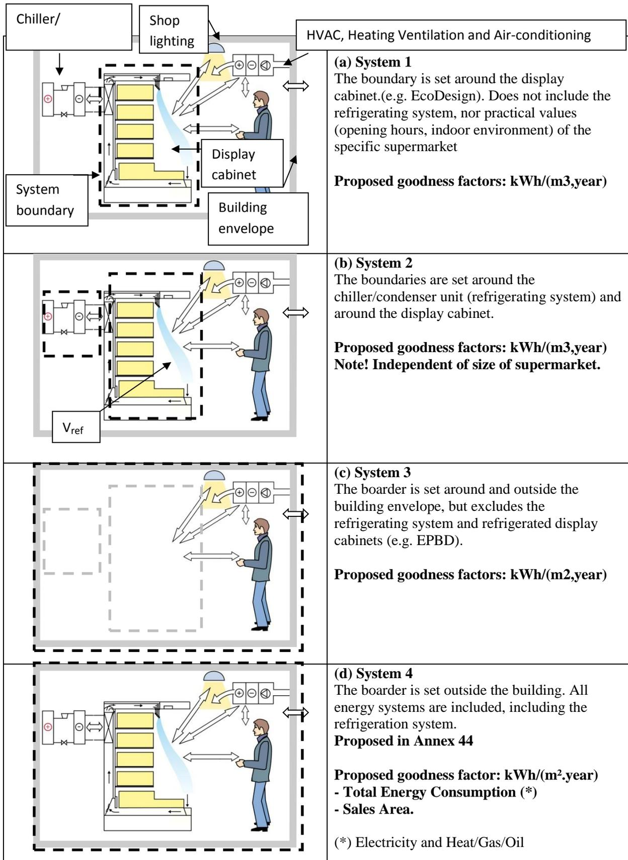
Figure 2. Illustrating four different options for system boundaries in a supermarket. ( from Lindberg, Axell and Rolfman 2011, ICR2011 ID 869). Figures (a)-(d) illustrate different system boundaries.
