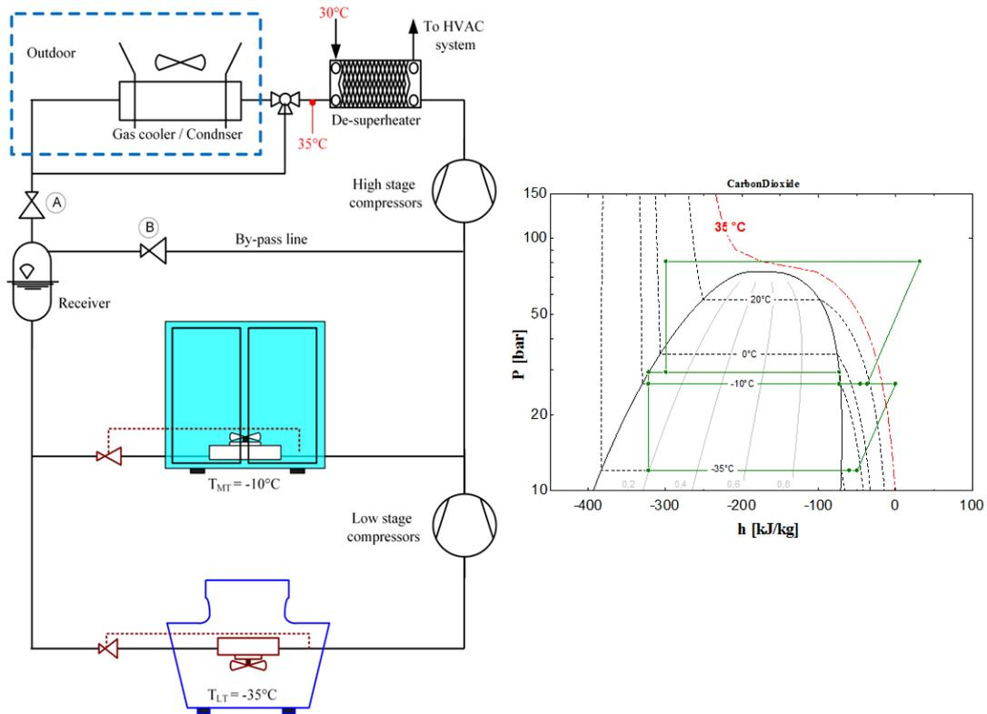
Figure 61: CO<sub>2</sub> trans-critical booster system schematic (left) CO<sub>2</sub> trans-critical booster P-h diagram (right)
