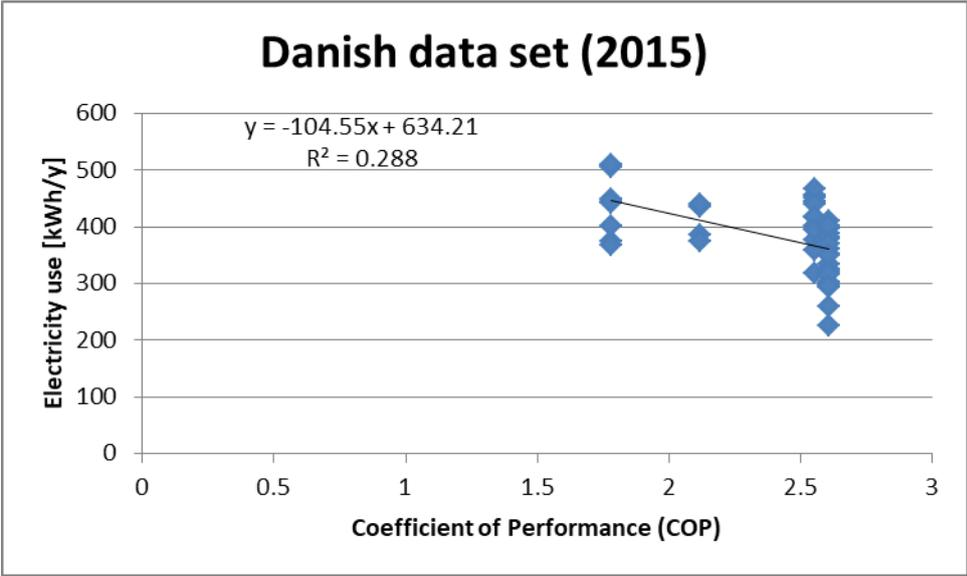
Figure 42: SCOP values calculated from nominal refrigeration demand and measured yearly energy consumption for refrigeration, for the Danish data set (2015), grouped per refrigeration system type
