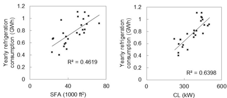
Figure 18: Correlations of refrigeration energy consumption with Sales Area (SFA) and refrigeration load (CL) taken with permission from the article by S. Acha (2016). Sample of 25 UK supermarkets (CO2 refrigeration systems only), cabinet loads evaluated at test conditions (25°C, 60% RH).
