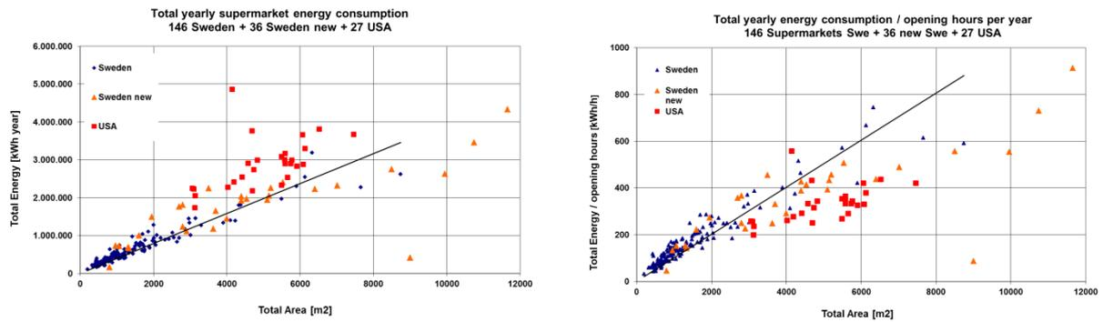
Figure 28 Total yearly energy consumption versus area (left graph) and total yearly energy consumption / (yearly) opening hour versus total area (right graph) for Sweden and USA (Annex 31, 2011).
