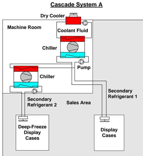
Figure 58: System Design 4: Cascade System (Arias, 2005)
