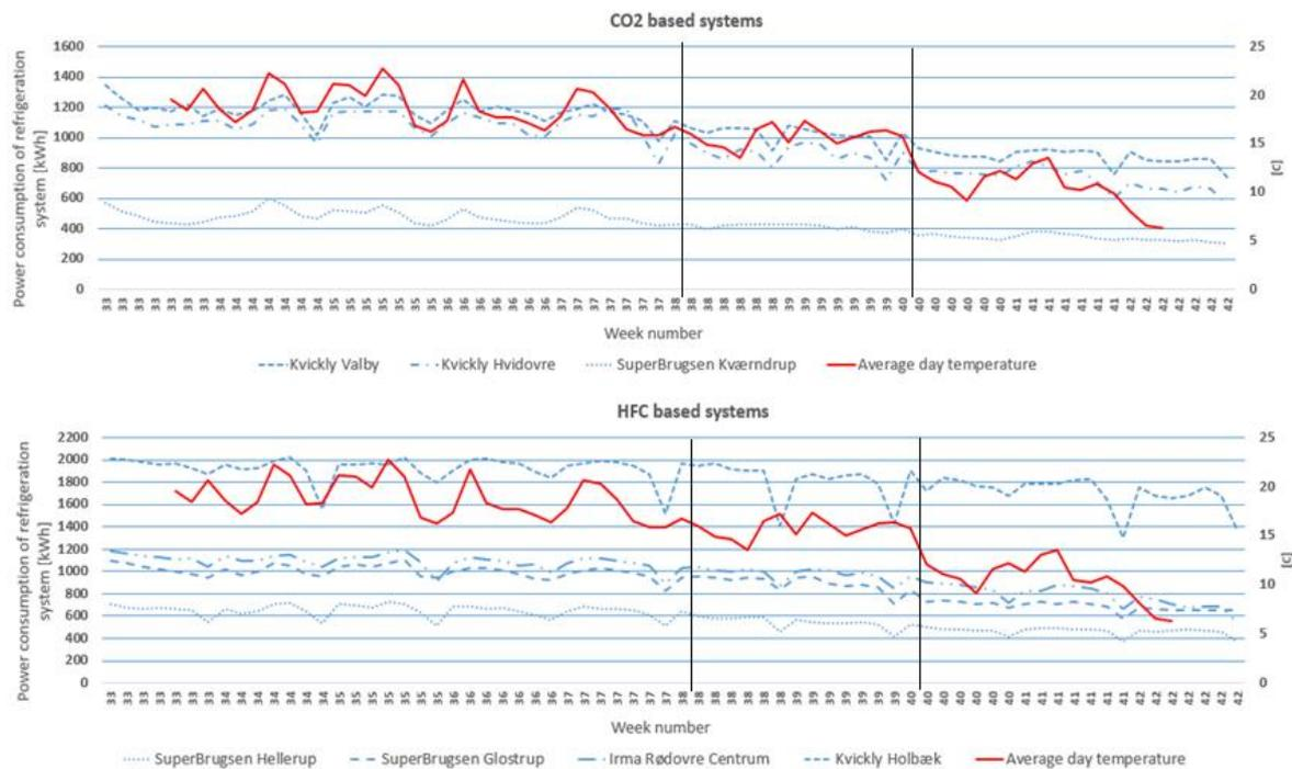
Figure 51: refrigeration energy consumption before, during and after the test period for CO2 based systems (above) and for HFC based systems (below).
