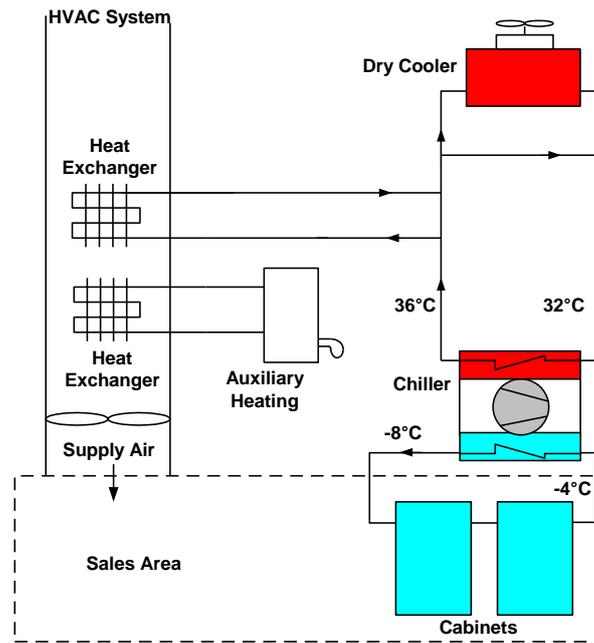
Figure 63: Heat Recovery System Design 3
