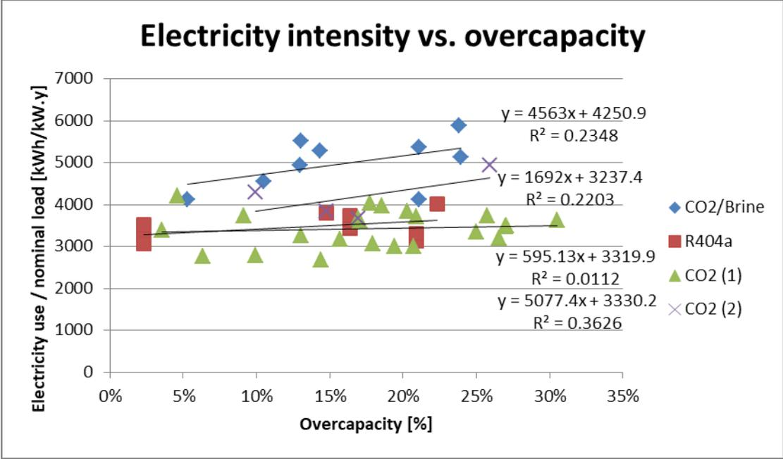
Figure 71: Refrigeration electricity use per kW of nominal load, as a function of overcapacity per kW of nominal load. Trend line functions in same order as legend
