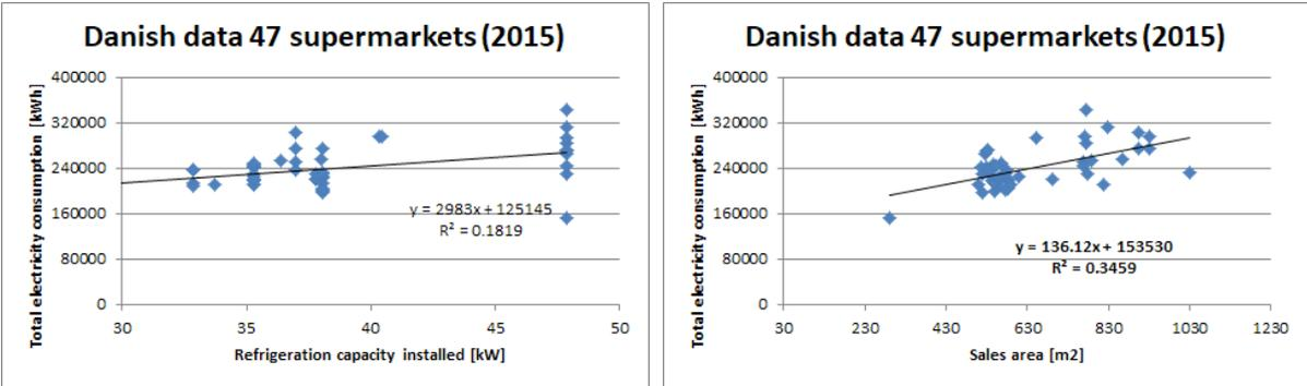
Figure 23: trend lines of total electrical energy consumption based on installed capacity (left) and sales area (right) for the Annex 44 Danish data set (trend lines not through origin but with intercept).
