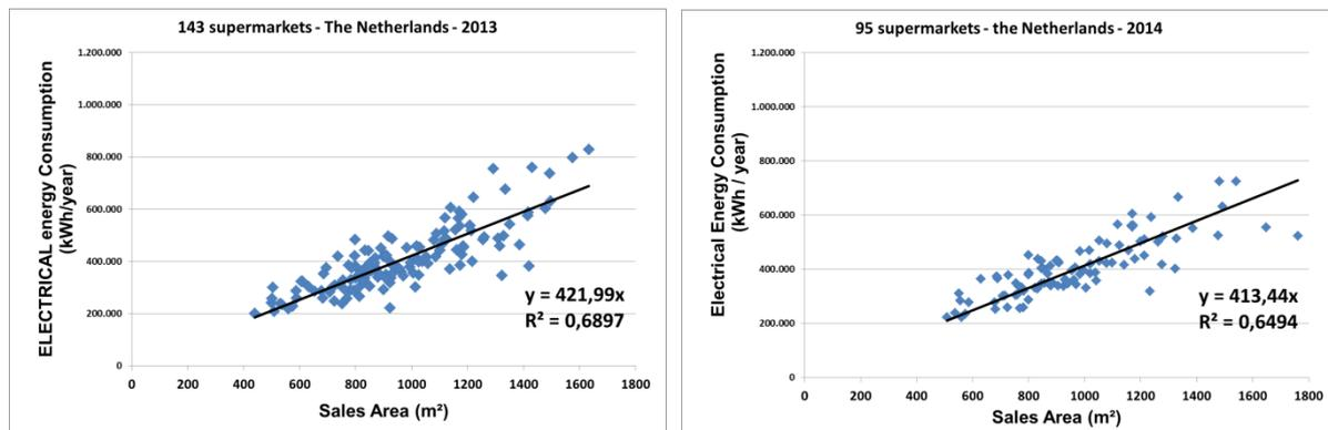
Figure 13: representation of the Dutch data sets: electrical energy consumption versus Sales Area (2013 and 2014).
