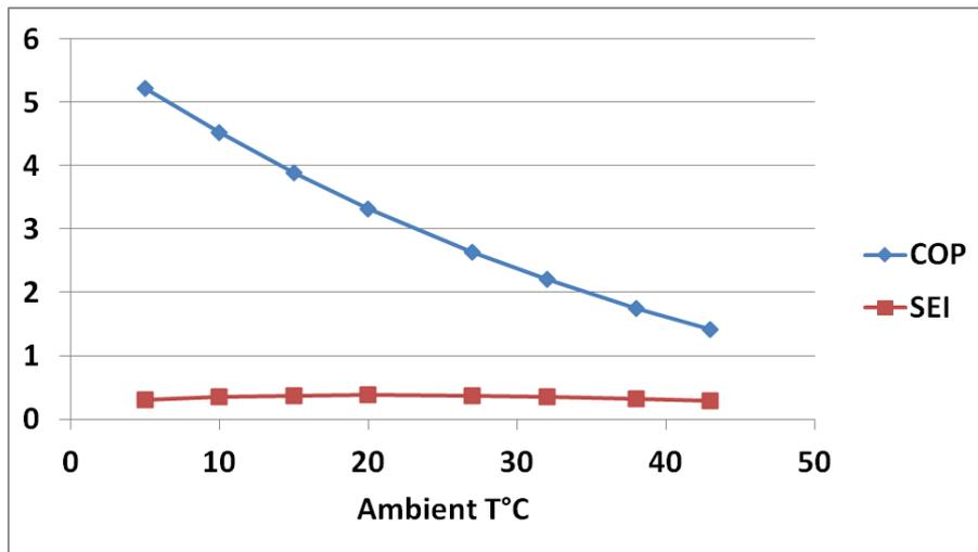
Figure 40: Theoretical values of COP and SEI based on manufacturer's data, using R404A, with fixed evaporation at -10 °C, and 20 °C suction gas temperature.
