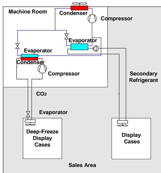
Figure 59: Cascade System with CO<sub>2</sub> in the Low Temperature Stage (Arias, 2005).
