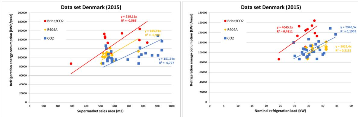
Figure 20: Correlations of refrigeration energy consumption with Sales Area and nominal refrigeration load for the Annex 44 Danish data set (2015) – with separate correlations for different refrigerating system types.
